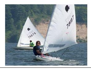
A race rigged Sunfish racing on Irondequoit Bay, NY. The rig is carried lower to the deck and additional lines are added to control sail shape
